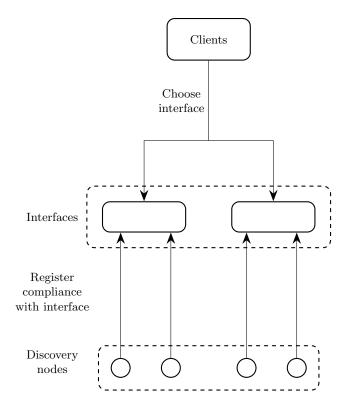
Figure 3: Discovery API interface registration and usage
